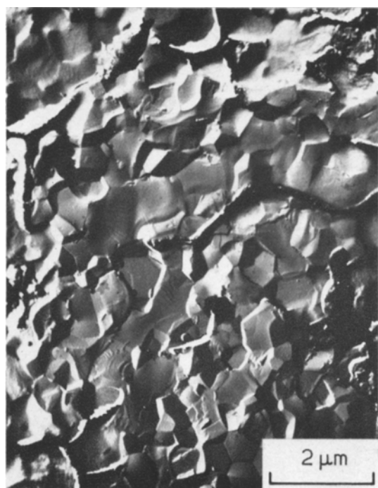
Figure 9 G78 heated at 900° C for 3 h. Replicas prepared after 5 sec etch with 0.1% HF.
